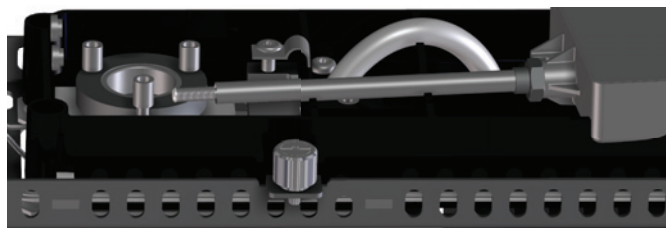
Figure 18 NPD collector, upper insulator, and metal C-ring
