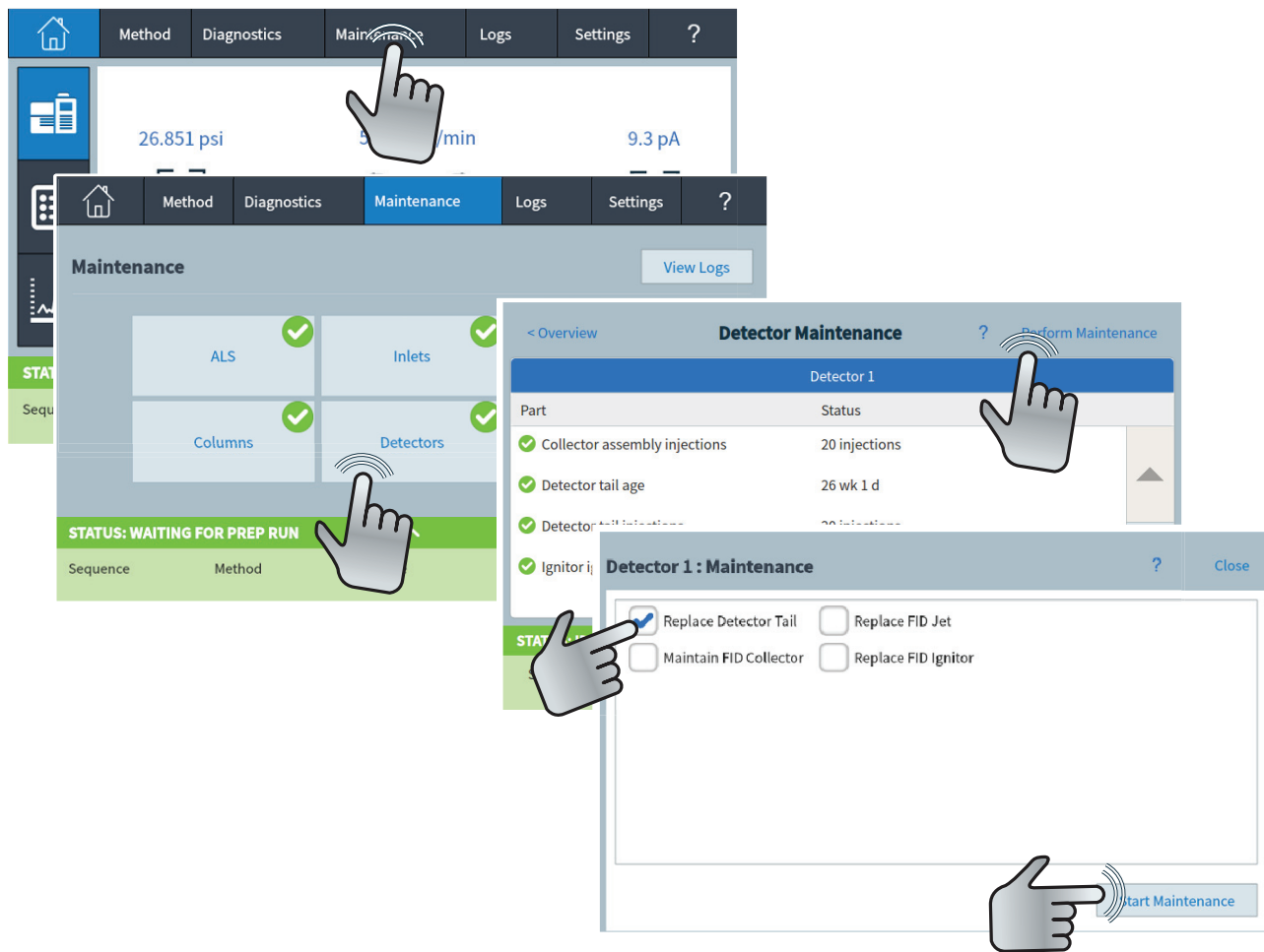
Figure 16 Launching the maintenance wizard
